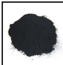
Carbon black is added during tire manufacturing and make up approximately 30% of the final product.
